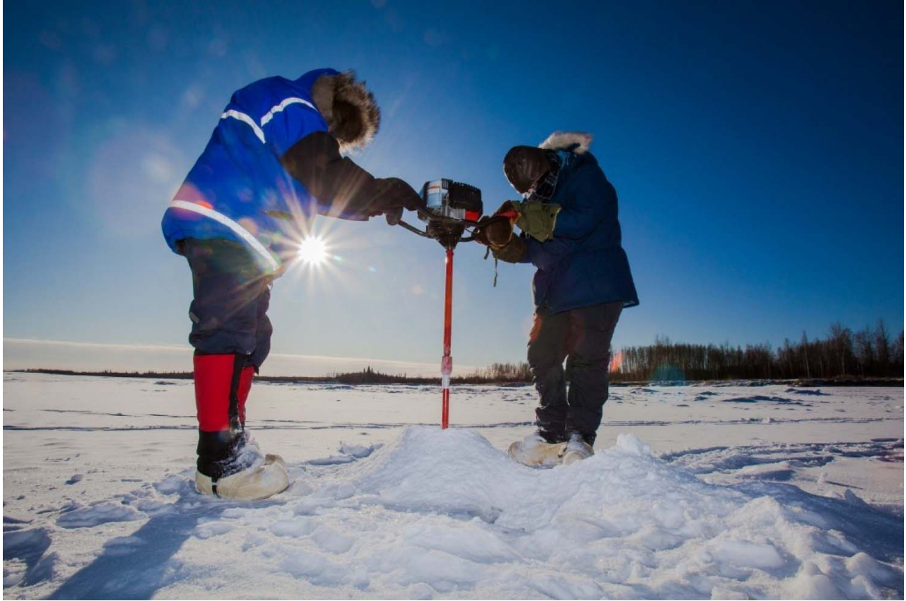
Researchers Jack Schmid, left, and Dominique Pride drill through the ice on the Tanana River near Nenana to determine its potential for placement of a hydrokinetic generator in this Feb. 26, 2010, file photo. (Todd Paris/University of Alaska Fairbanks)
